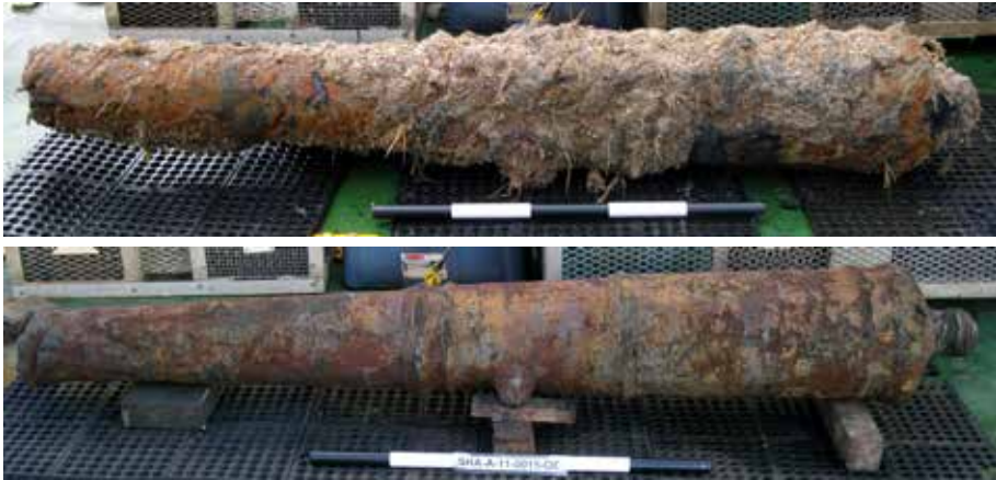
Figure 4. Gun C13 from Site 30E, a possible English saker ordinary iron gun before and after the removal of concretion (length 2.43 metres, SHA-A-11-0015-OE).
